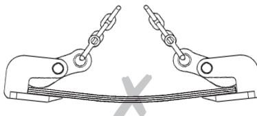
It is forbidden to apply lateral tensile forces with an inclination angle of more than 15° to the load lifting attachment.
