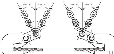
Any modifications of the load lifting attachment are prohibited.
