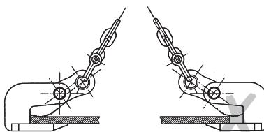
Do not use the base frame for lifting further load lifting attachments or for attaching loads by means of ropes, belts or chains.
