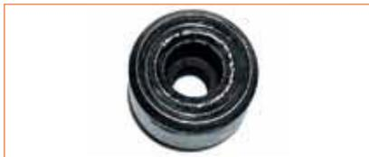
interior ring damaged for 100%
