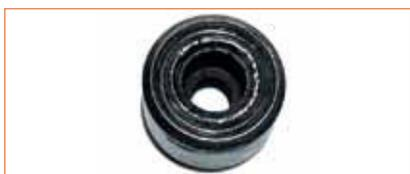
interior ring damaged for 100%
