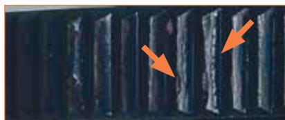
1 complete teeth not sharp and 1 damaged
