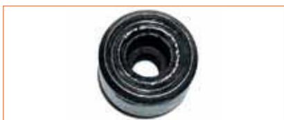
interior ring damaged for 100%
