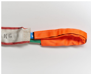
Figure 1: Slings before and after replacing
