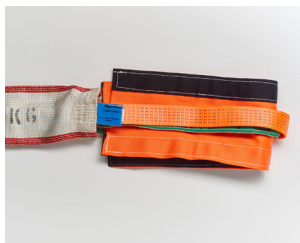
Figure 3: Protective sleeve with U-shaped position in loops
